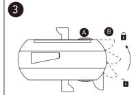
Rotate adaptor lock **B** clockwise 90° to connect the adaptor to the neutral circuit.
